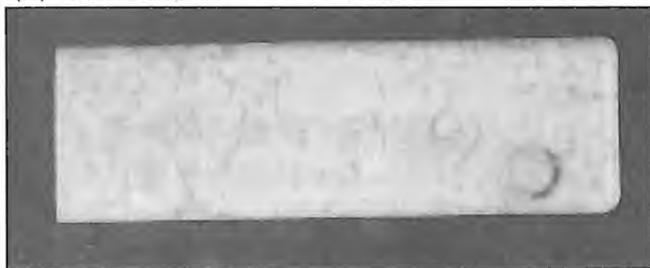
(b) 低強度  $\sigma_f=12.35\text{MPa}$ ,  $K_{IC}=0.66\text{MPa}\cdot\text{m}^{0.5}$
